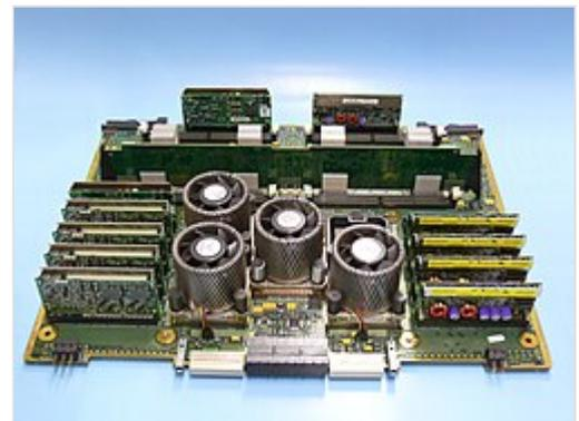
HP 9000 RP7410 system board with quad PA-RISC 8700+ CPUs
