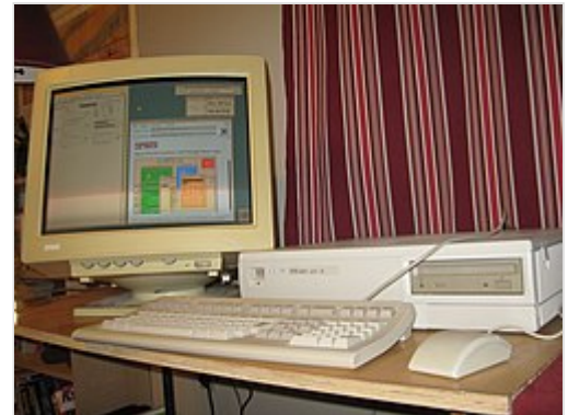
VAXstation 4000 model 96 running OpenVMS 6.1 and DECwindows
